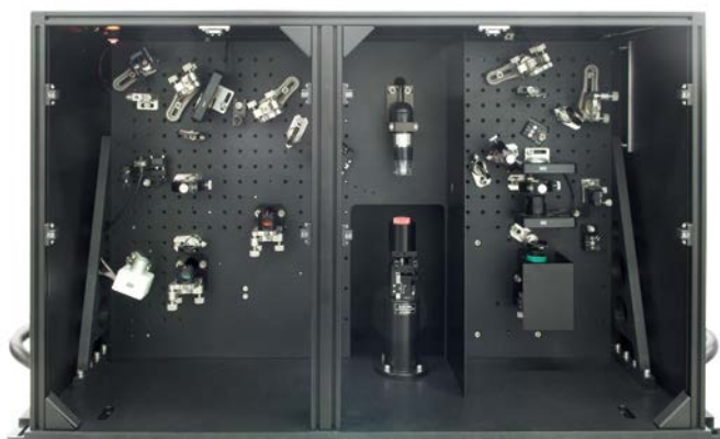
Standard layout of the vertically-arranged sample compartment of the SFG spectrometer
