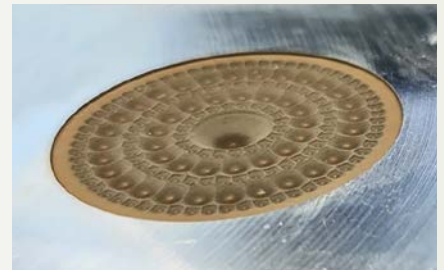
Textured aluminum molds. Courtesy of FTMC.
