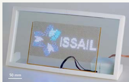
SSAIL technology on PA4T. Courtesy of Akoneer.
