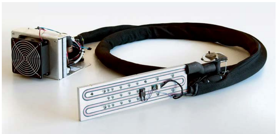
A cooling plate is attached to the laser on one side of the design (above). On the other, a compressor with auxiliary electronics is installed into the laser power supply unit.
