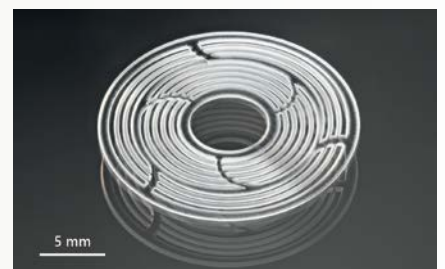
Thin fused-silica cutting. Courtesy of FTMC.
