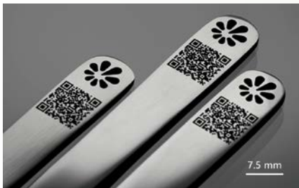
Black marking of tweezers. Courtesy of FTMC.
